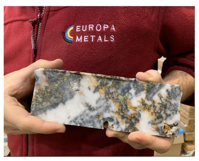
TOD-020 drill core with highly visible chalcopyrite copper sulphide mineralisation
