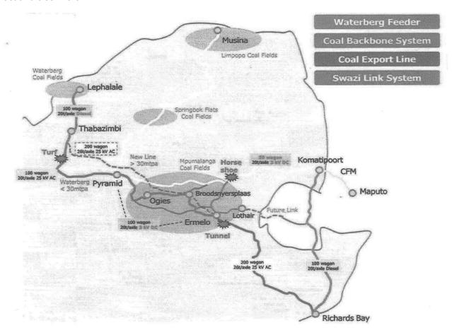
Figure showing Proposed Rail Upgrades to Waterberg Coal Sources (source: Transnet 2012)
