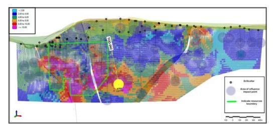
The cross section image above illustrates the positioning of hole TOD-042. The high grade nature of the intersection is consistent with our current resource model and provides further support for extending the known estimated indicated resource at that depth.
