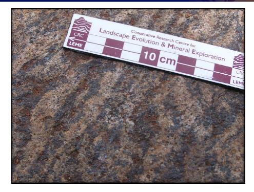
Figure 1: Coarse grained quartz magnetite gneiss, characteristic of the Moonlight mineralization.
